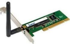
A green PCI wireless network card with a metal mounting bracket and a gold-plated PCI edge connector. It has a small antenna protruding from the top of the card.                                                                    |
