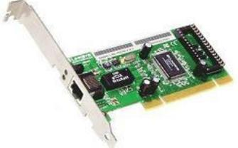
A green PCI Ethernet network card with a metal mounting bracket on one side and a gold-plated PCI edge connector on the other. It features a BNC connector for coaxial networking and an RJ45 port for standard Ethernet networking. |
