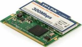
A green MiniPCI wireless network card. It is a smaller version of a PCI card, designed for use in laptops. It has a gold-plated MiniPCI edge connector and a small antenna.                                                        |
